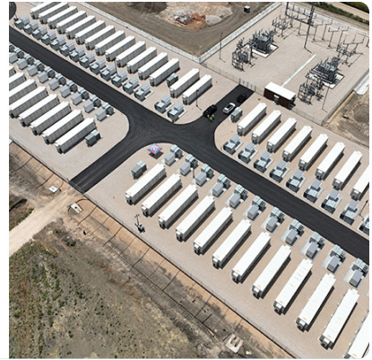
BESS at various scales: A residential on-site BESS, a small off-site BESS with 20 MW in New York, and a large off-site BESS with 100 MW in Texas. (Photos: SunPower; Key Capture Energy)
